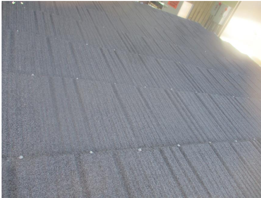
Specimen No. 1 After Testing – No Failure
